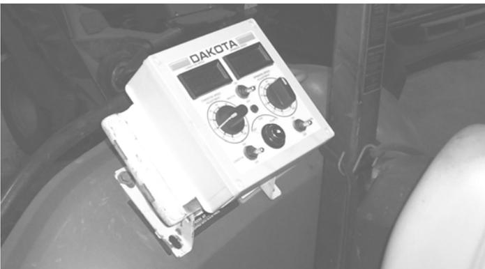
The mounting bracket for the control box is to be mounted in a position convenient for the operator (either on the right rear fender, on the dash, or to the roll bar of the tractor). Select a location for mounting the bracket making sure you will be able to remove and install the control box from the bracket without interference. To mount the bracket to the fender, use the following procedure:
