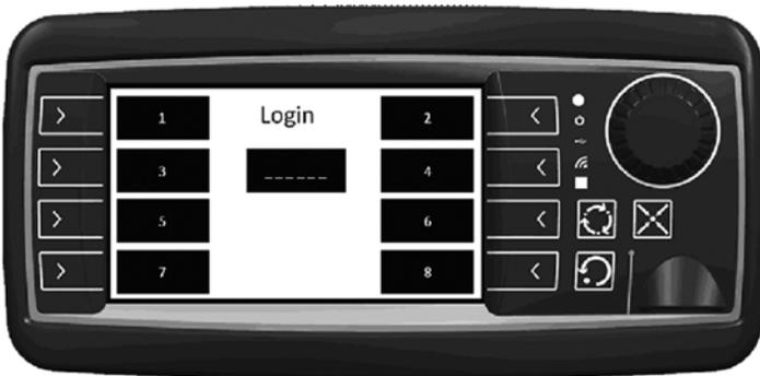
The Login screen will show when the Login button is pressed from the Menu screen. The Login screen is to be used to access either the OEM Setup or the Calibration screens. Entering the appropriate password will access the desired screen. If the password is entered incorrectly, the Login page will reset.
