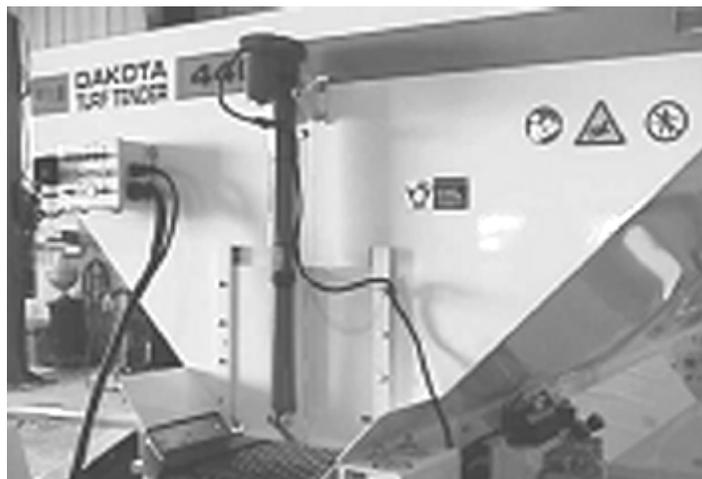
The electric front gate is easy to operate. One switch moves the gate either up or down. Push the switch away from the tractor operator and hold to open the gate. Pull the switch toward the operator and hold to close the gate. Releasing the switch will stop the gate at whatever position it is in.
