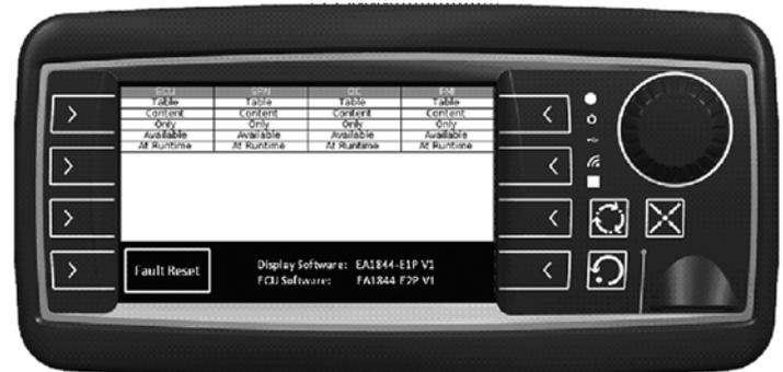
When a fault has been indicated by the fault icon, press the fault button to bring up the fault code table to identify which function is experiencing a fault. Troubleshoot the wiring to the function according to the fault code table. When the fault has been corrected (usually a broken wire, loose connection, or wire grounding on the frame), then press the Fault Reset button to reset the fault.
