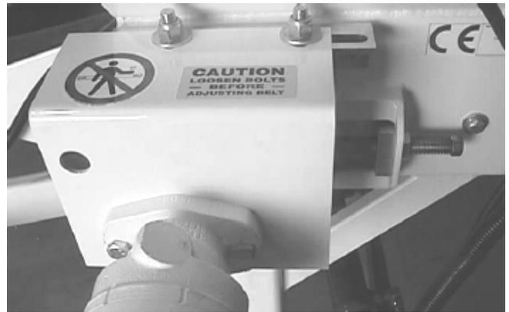
3. Using a  $\frac{3}{4}$  inch wrench, turn each tensioning bolt clockwise 1-2 complete turns. Be sure to make equal adjustments on both sides.
