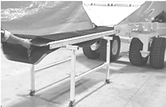
8. Roll the belt run over on its side and remove the old belt from the belt run.
