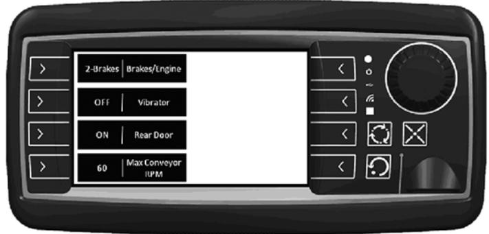
The OEM Setup screen is used to change the machine settings.
