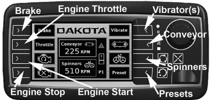
**BRAKE** Applies the brakes for a period of 2 seconds.. The GAIN of the brakes may be adjusted in the menu screen and the brake adjust button is pressed; then use the ENCODER dial to adjust the GAIN. The GAIN adjustment range is from 10% - 100%.
