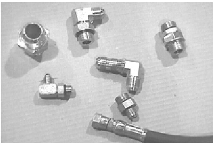
All components use either an O-ring boss or 37° flare hydraulic fittings. Do not use pipe-threaded hoses or fittings for replacements. Do not use Teflon tape or pipe thread compound. These are not helpful and may cause damage to the system.
