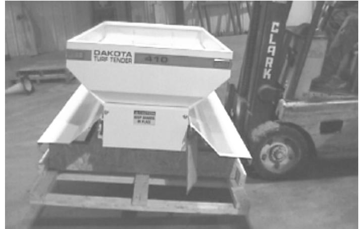
2. While wearing gloves and safety glasses, hold the longest free side of each band; then carefully cut each of the bands (as close as possible to a corner) securing the hopper to the skid.
