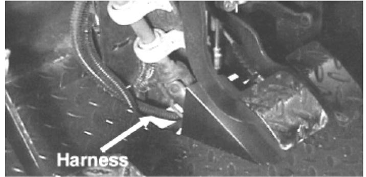
4. Place the control box bracket in the desired mounting location (within easy reach and view of the operator) on the dash making sure there are no electrical wires in the area (below the dash). Using the bracket as a template, mark the location for the four mounting holes; then center punch the holes.
