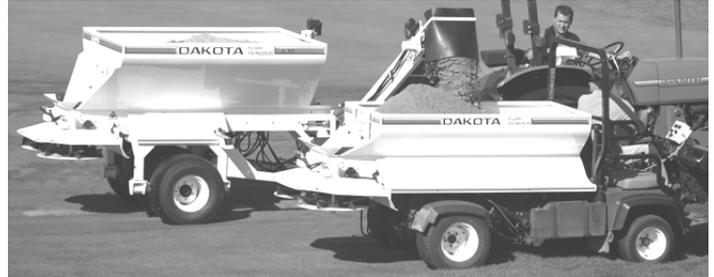
There are two positions for the side conveyor. The **traveling position** is when the side conveyor is retracted and rests against the side of the hopper. The **operating position** is when the side conveyor is fully extended to the side.
