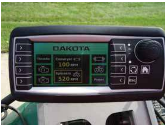
Can start/stop/throttle up and down the engine on units equipped with a power pack
