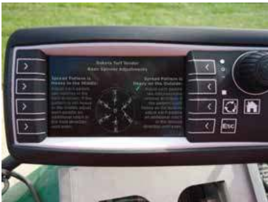
Reference guide for adjusting spinner paddles
