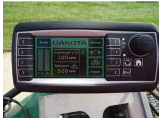
Control brakes and vibrator on equipped units
