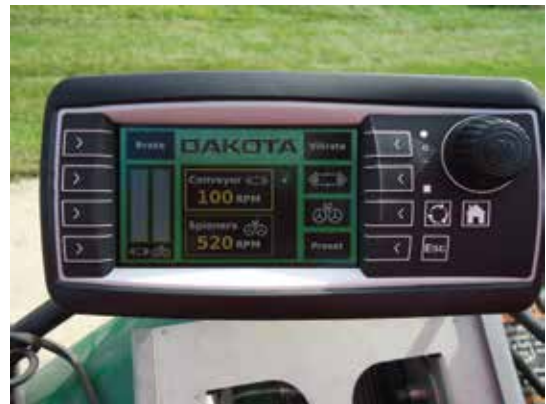
Control brakes and vibrator on equipped units
